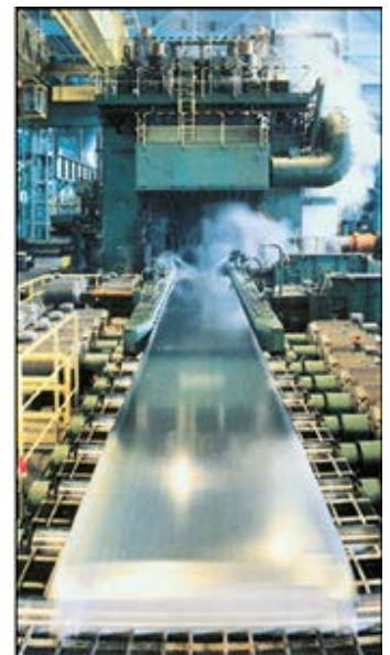
Aluminum hot rolling process using Rotary Brushes for several operations.
